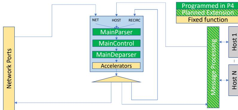
**Figure 1.** Programmable NIC Architecture Block Diagram
